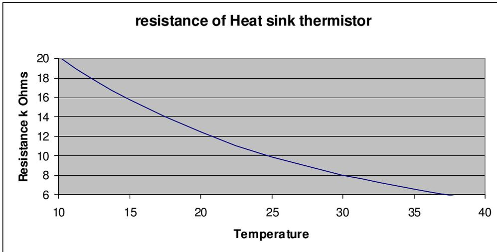
Alternatively the sensor can be tested while still connected to the PCB measure the DC voltage across the resistor and check it against the graph below.
