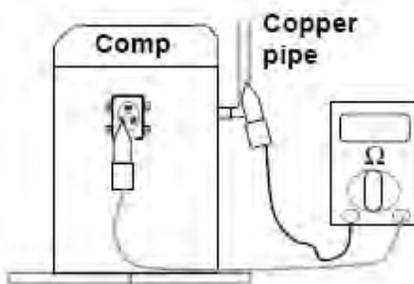
The next test is to measure the resistance of the compressor windings to earth. Using a Megger (high Voltage meter) measure the resistance from any of the 3 compressor terminals to an Earth point (pipe work). The value should exceed 2 M Ohms.
